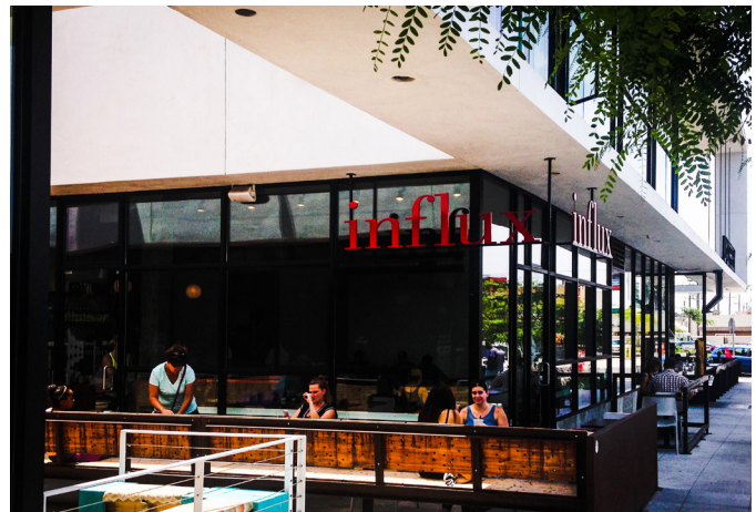
Differentiate first floor from upper levels to provide changes in massing. Articulate the street wall by incorporating plane changes and outdoor areas.
