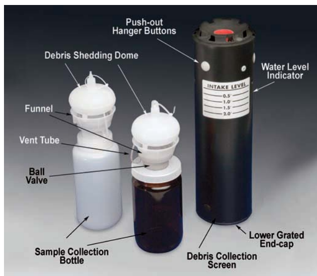
Figure 2-1. Nalgene First Flush Sampler Product Diagram
