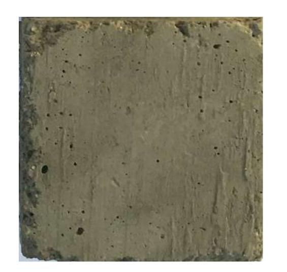
CAST IN PLACE CONCRETE BOARD FORM
