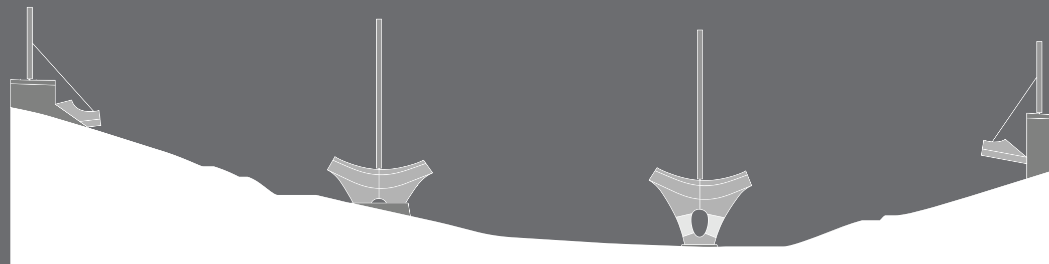
Stage 4: Primary pier components and temporary cable stay towers installed. First abutment components are installed and supported by temporary cable stays.
