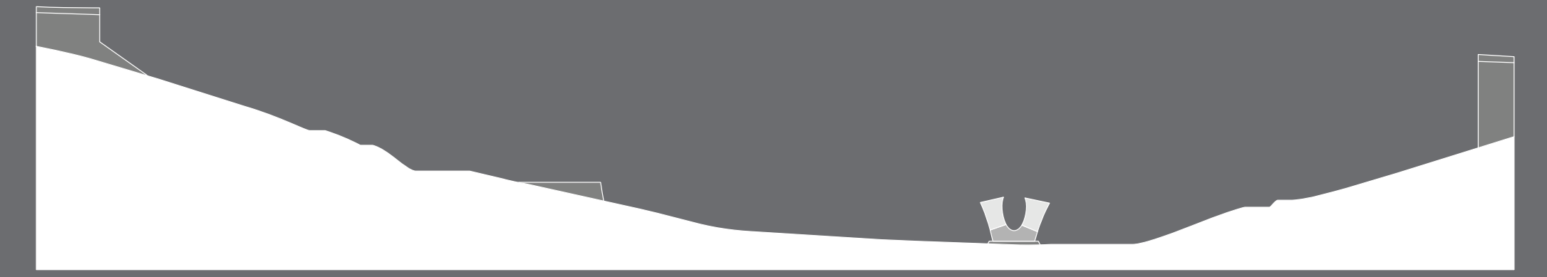
Stage 3: Second lowest east pier component installed.
