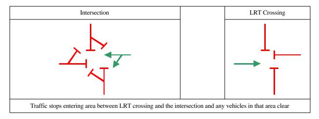
Figure 3: Sequence of Controller Operation, LRT Approaching
