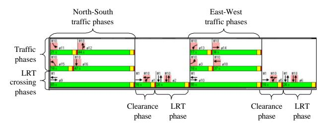
**Figure 7: Timing and Phasing Operation**
