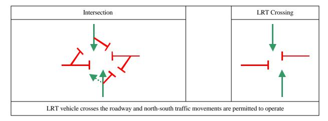
Figure 4: Sequence of Controller Operation, LRT Crossing
