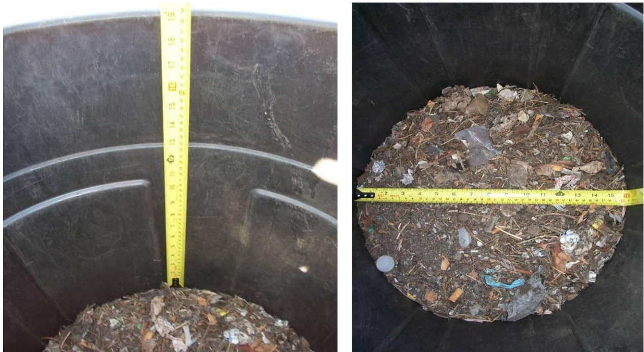
Figure 3-3. Measurement of Freeboard Depth and Diameter for Gross Solids Volume Calculation
