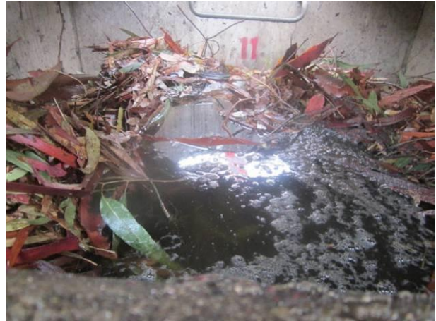
b) Product full of water and draining slowly at end of monitoring period.
