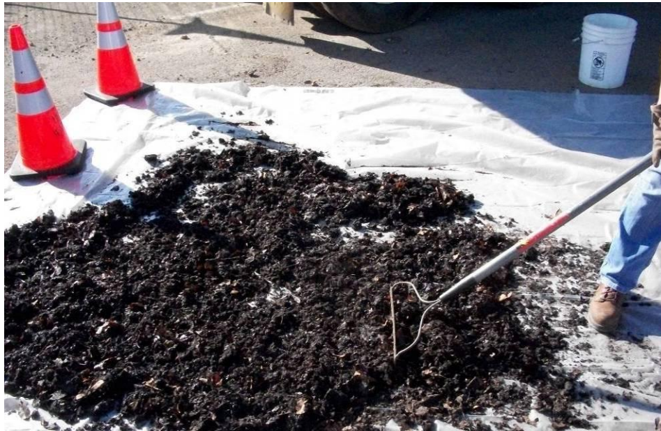
Figure 3-2. Drying of Gross Solids
