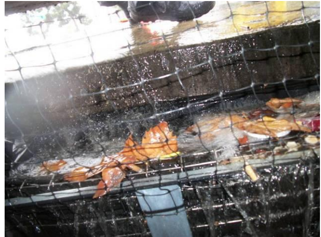
b) Flow bypass of BMP; smaller gross solids are re-suspended and bypass, larger gross solids retained by webbing.
