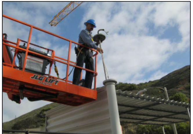
Photo 4-5: Transducer is Placed in Test Cylinder
