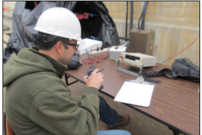
Photo 4-9: Water Level and Fluke Meter Readings are Radioed to Operator
