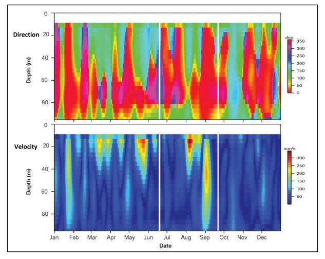
Figure II.B-3 Current Velocity and Direction by Depth at the PLOO, 2013 Data from PLOO outfall 100 meter station for 2013.
