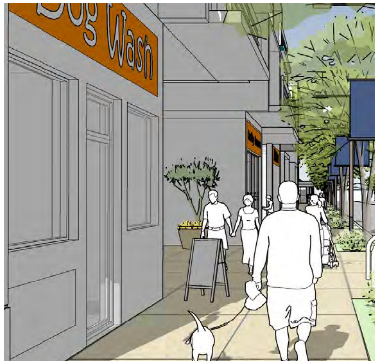
Create a sense of definition and enclosure by incorporating a consistent building setback ("street wall") within the Frontage Zone.
