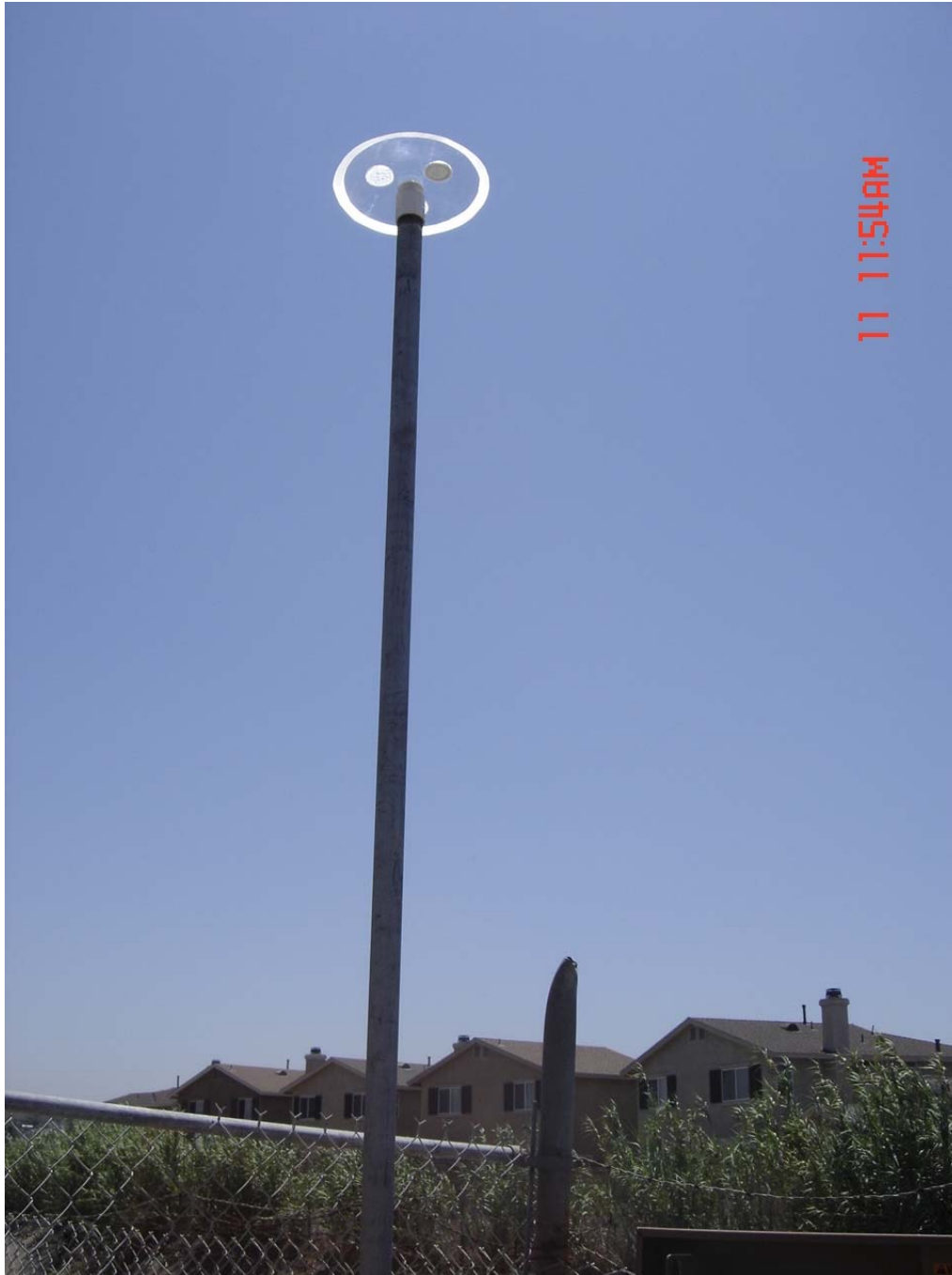
Figure 4-8. Aerodynamic deposition plate mounted on the rain gauge pole at site DPR(2)
