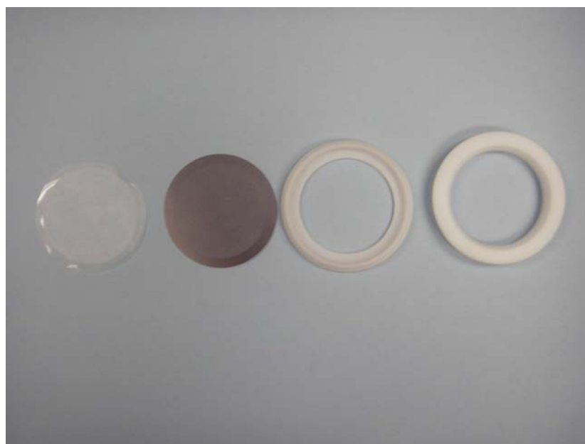
Figure 4-5. Teflon sample disk (left), and passive sampler cassette parts, backing screen (second from left), base (second from right), and top (right)
