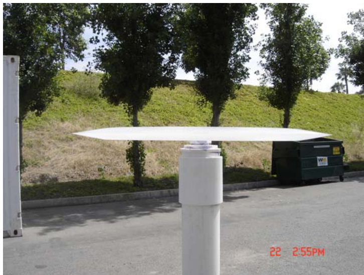
Figure 4-2. Cross sectional view of the aerodynamic deposition plate. Leading edge is at an angle of 10 degrees.
