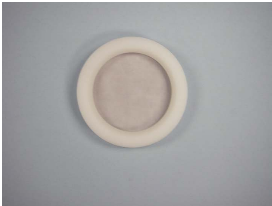
Figure 4-1. Surrogate sample disk cartridge
