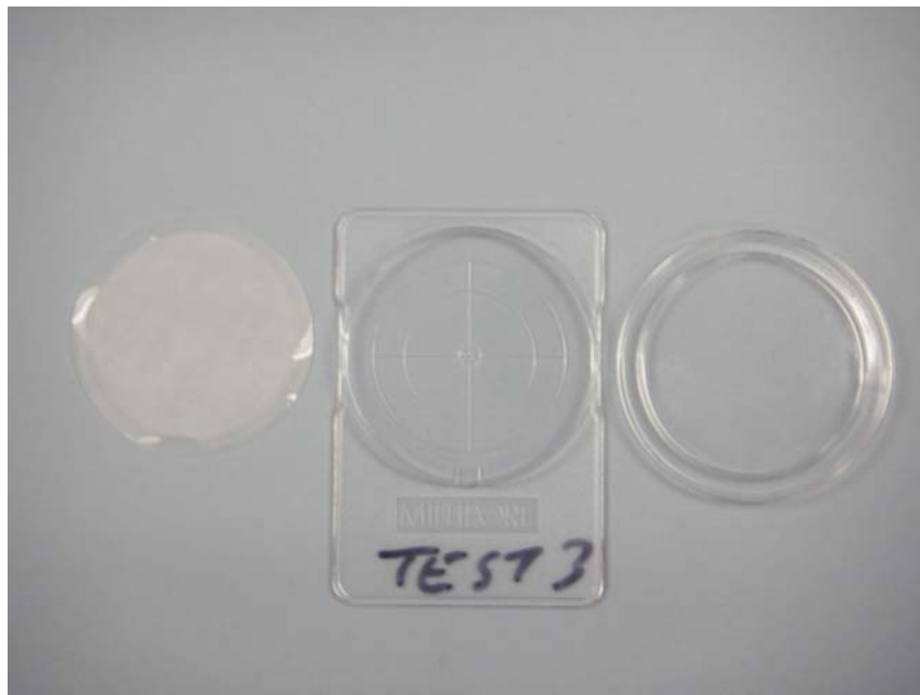
Figure 4-4. Teflon sample disk (left), shipping cartridge (middle), and cover (right).
