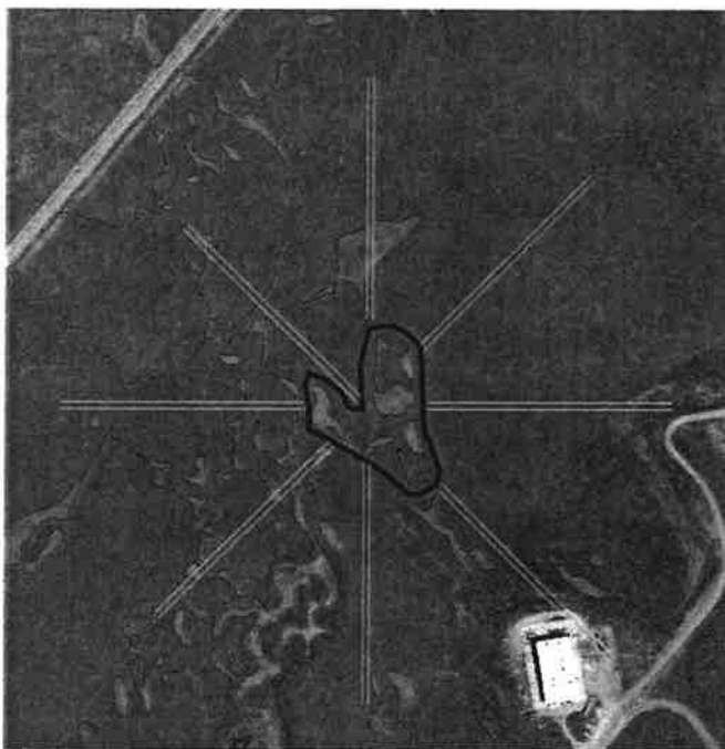
Figure 5. Example of the method used to estimate Buffer Width. Note that the width is based on the lengths of eight lines A-H that extend at regular intervals around the perimeter of the AA where buffer is present. If a portion of the perimeter of the AA does not have buffer that is at least 5 meters wide, do not place a line there.
