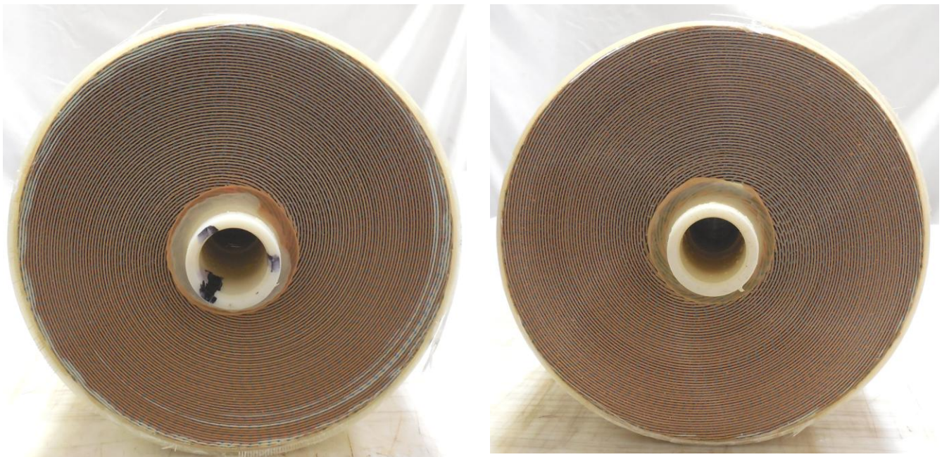
Image of feed scroll end (left) and concentrate scroll end (right) for SN# SOY35015
