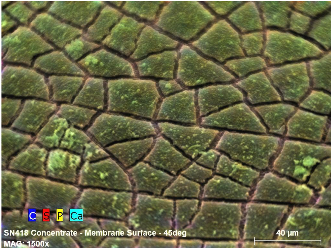
CEI image (1500x) of the membrane surface on the concentrate end
