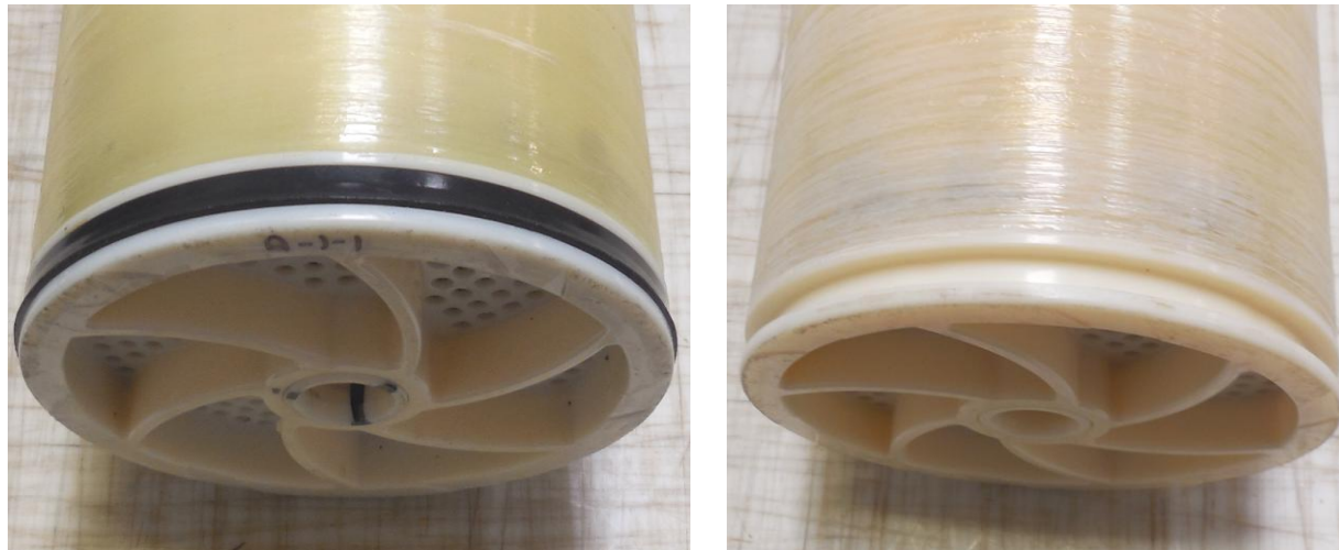
Image of feed ATD (left) and concentrate ATD (right) for SN# SOY35615
