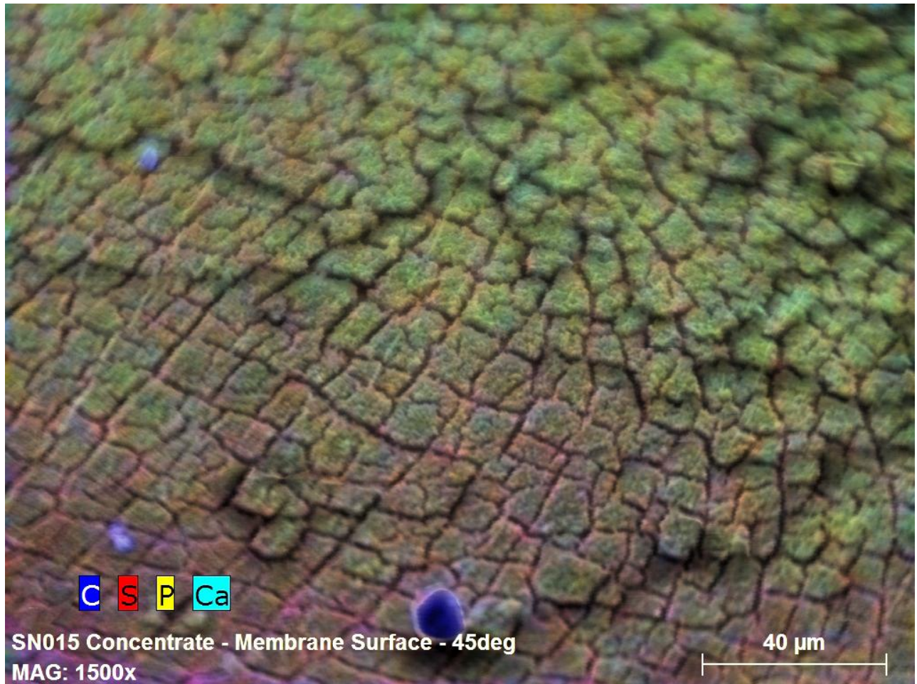
CEI image (1500x) of the concentrate end of the membrane surface
