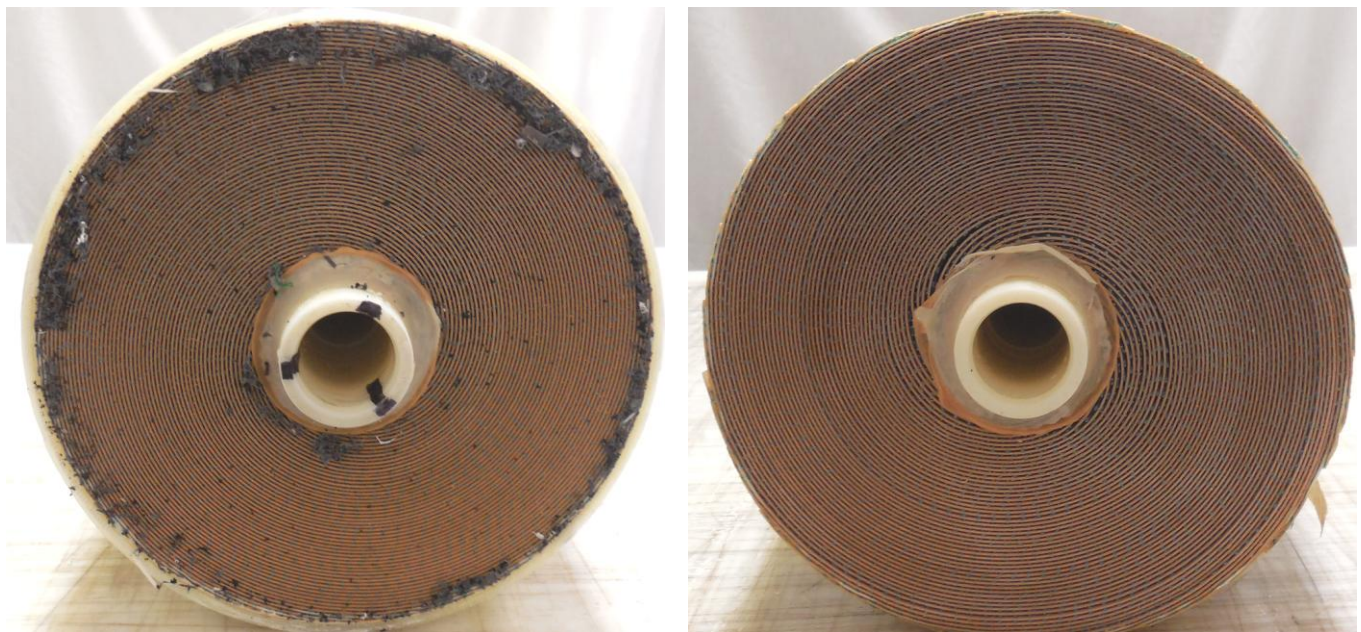
Image of feed scroll end (left) and concentrate scroll end (right) for SN# SOY35615
