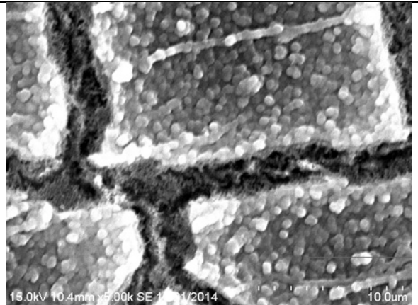
Figure 4.6. SEM micrograph of S/N 100930418 membrane at magnification of x5,000.
