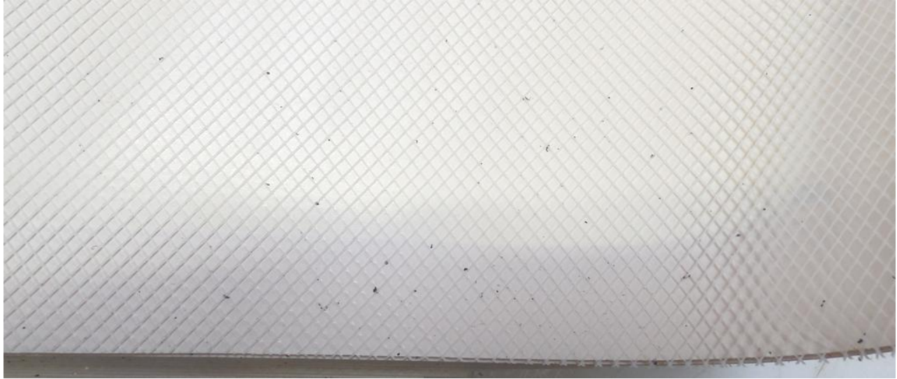
Image of particles observed on the feed end of the element
