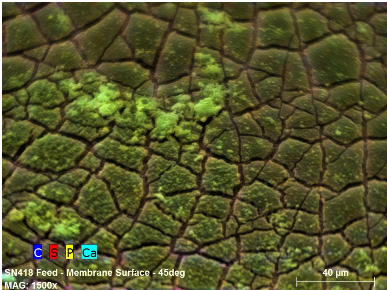
CEI image (1500x) of the membrane surface on the feed end
