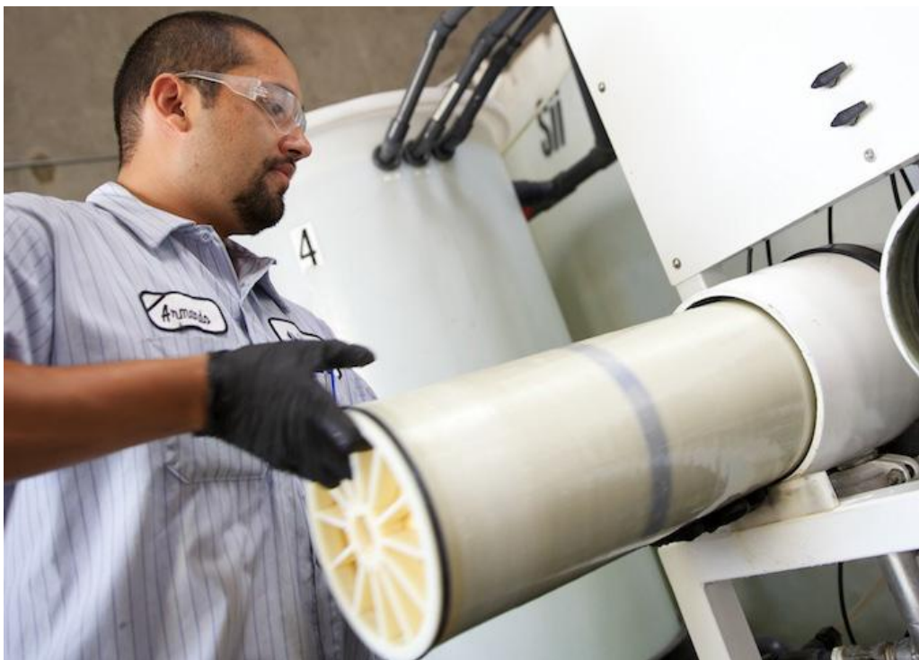
Element Wet Testing
