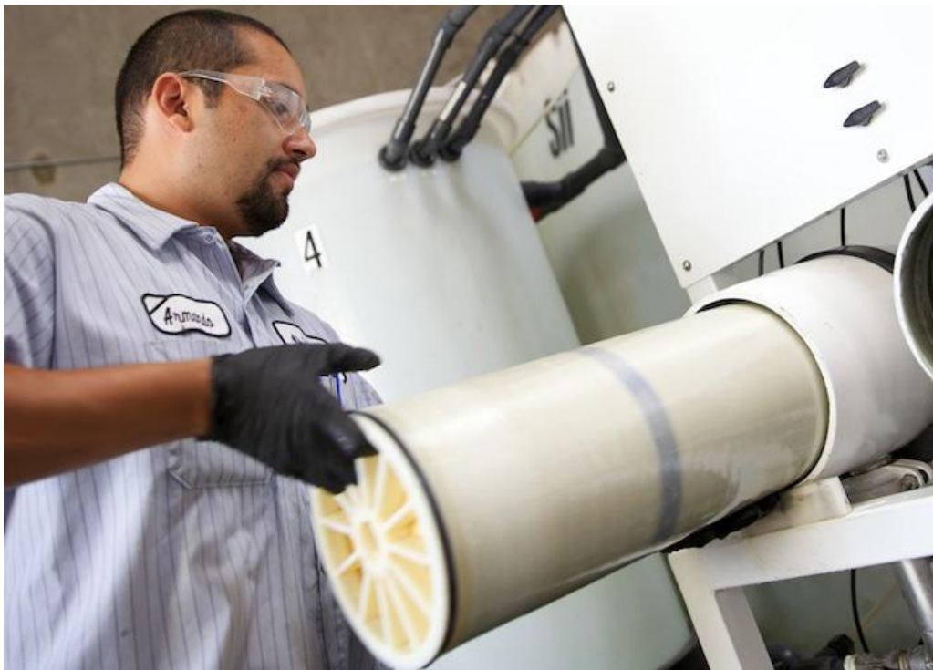
Element Wet Testing
