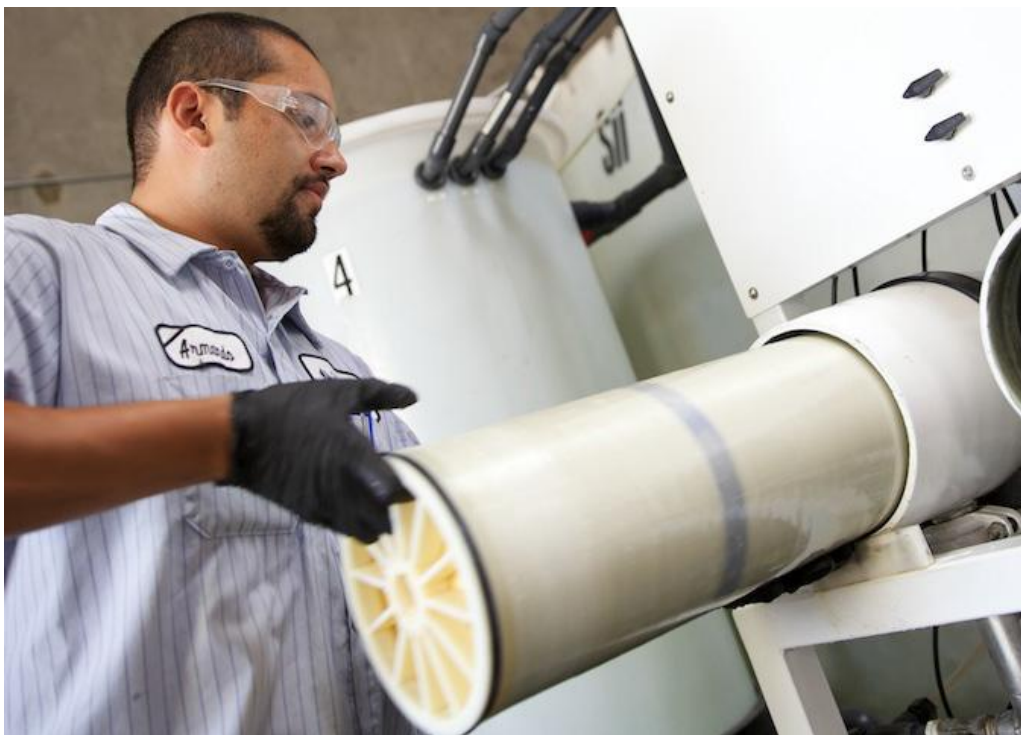
Element Wet Testing
