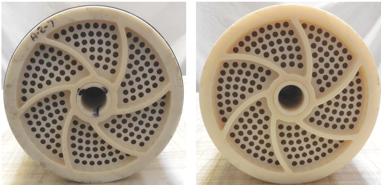
Image of feed ATD (left) and concentrate ATD (right) for SN# SOY35015
