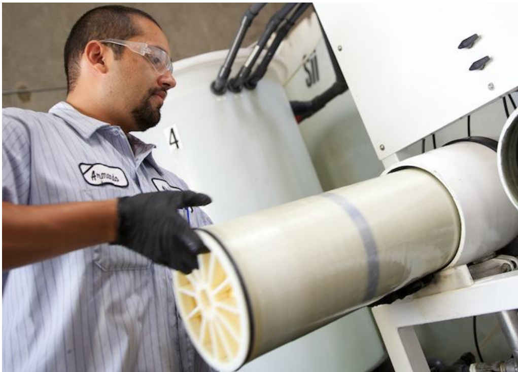
Element Wet Testing
