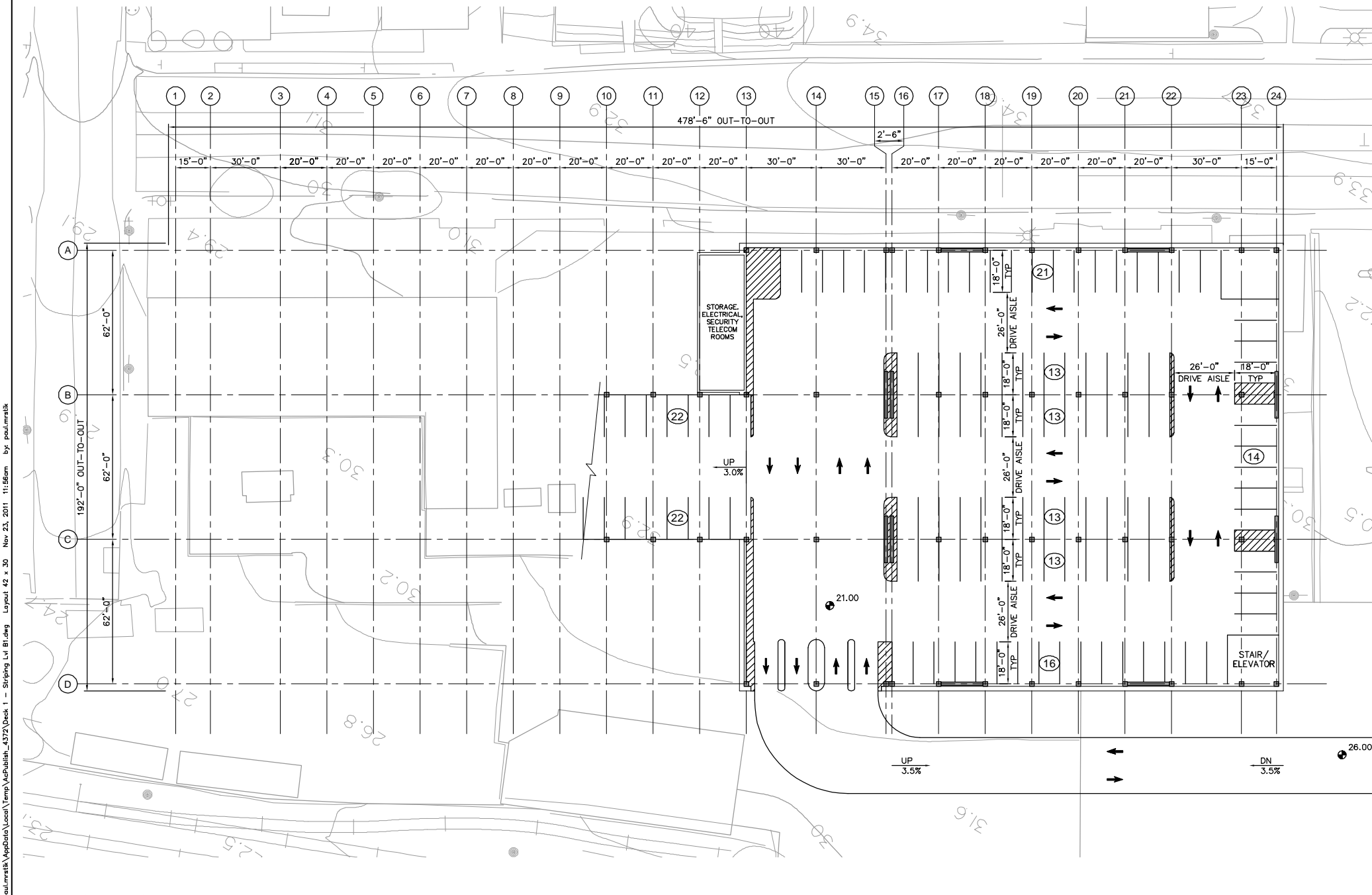
1 STRIPING PLAN - LEVEL B1 SCALE: 1" = 20'-0" TR101
