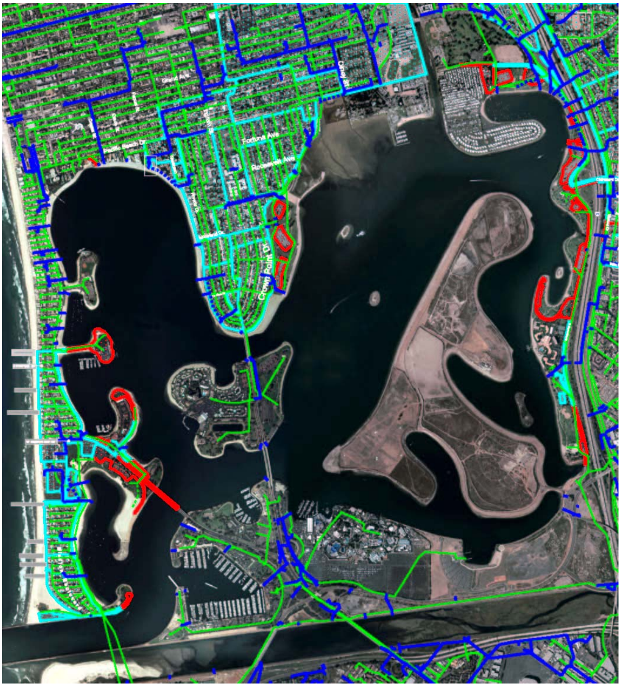
Figure I-4. Map of Mission Bay storm drain diversion system showing diverted areas in blue and un-diverted areas in red.
