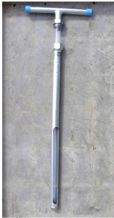
Push core soil probe with sterile butyrate liner
