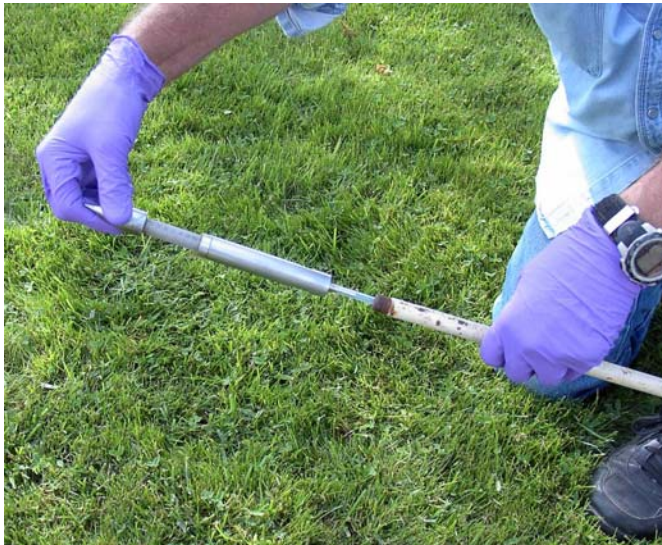
Beach spring groundwater sampler showing screened, retractable sampling port
