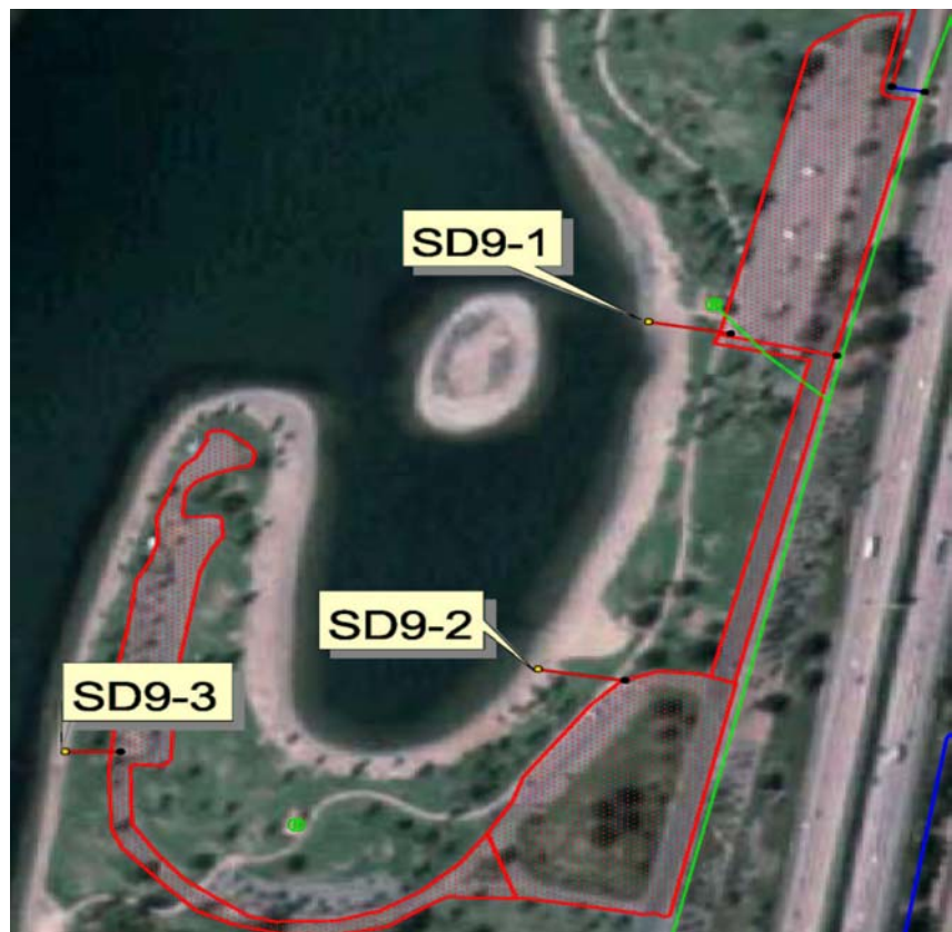
Figure I-26. Map of storm drain system at Leisure Lagoon showing diverted (in blue) and un-diverted areas (in red).
