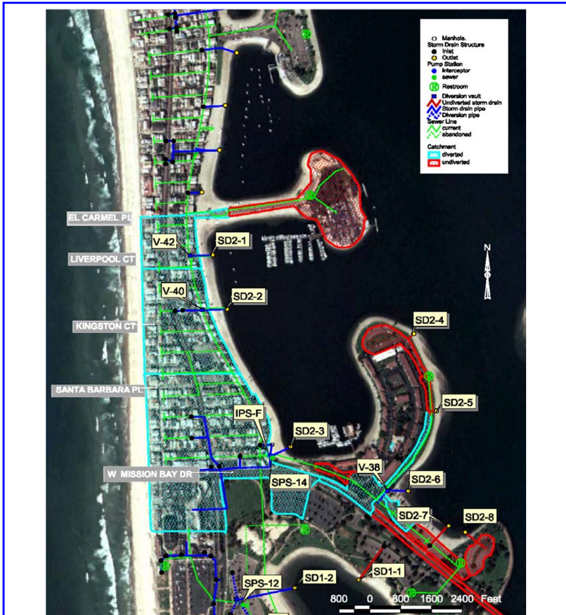
Figure I-9. Map of storm drain system at Bahia Point showing diverted (in blue) and un-diverted areas (in red).
