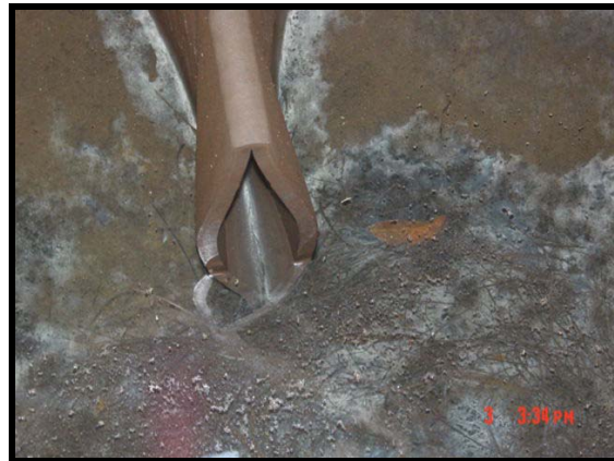
Figure I-8. Broken Bonita Cove tide flex valve stuck open.
