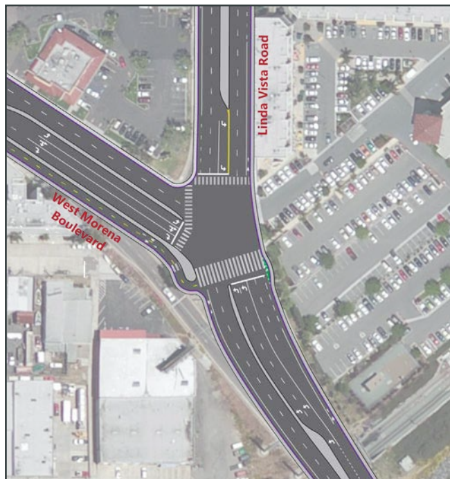
Figure 3-8 - Proposed Intersection Conceptual Design for Improvement 6
