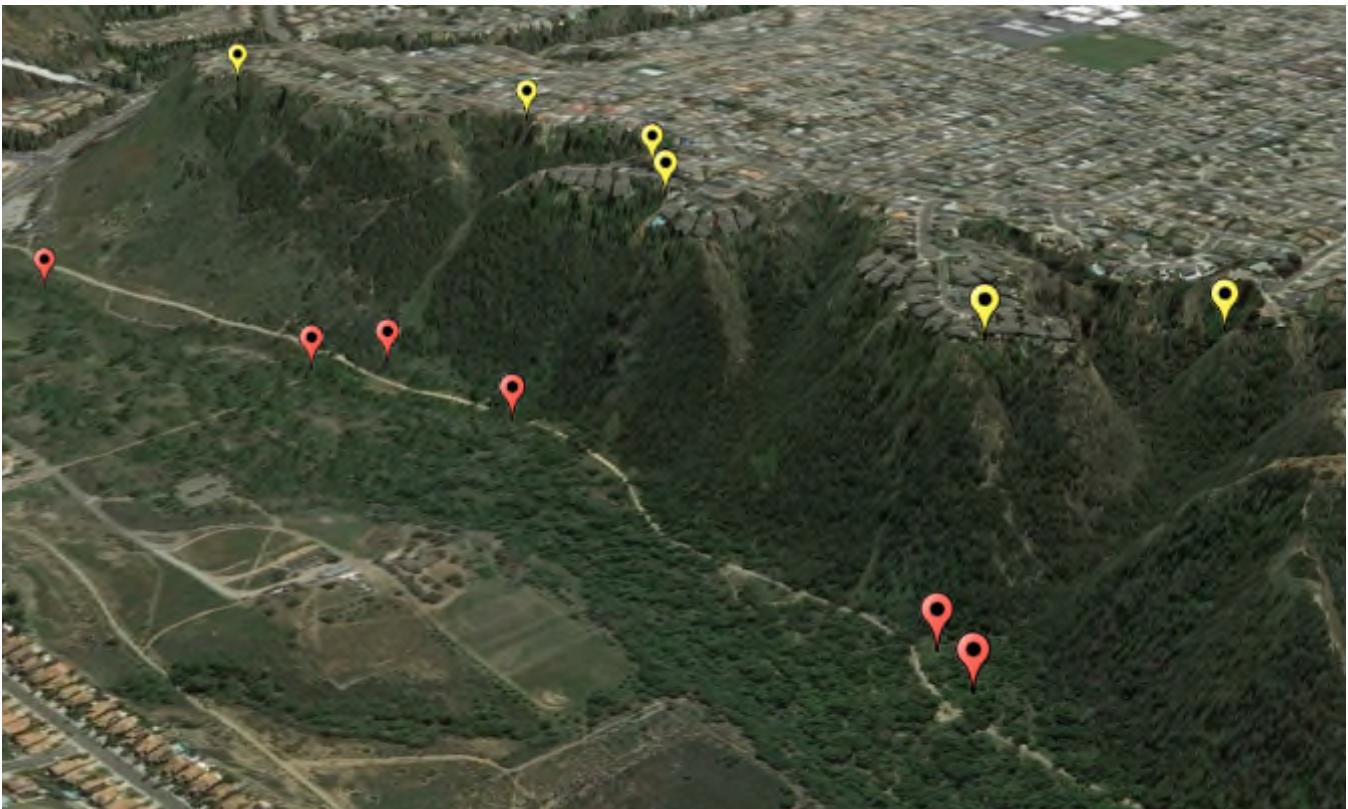
Figure 4-1 Existing outfalls (yellow) physically moved to valley floor (red).
