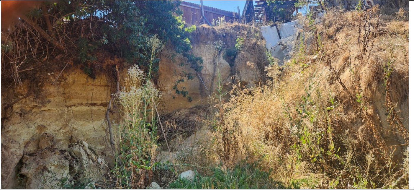
Looking west at artificial fill within the vertical back scarp of the ravine.
