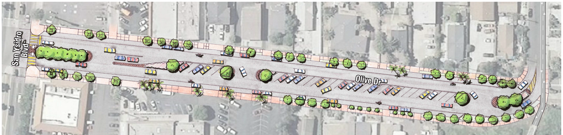
Example streetscape in plan view, featuring traffic calming, landscaping, crosswalks, and connection to the pedestrian bridge.
