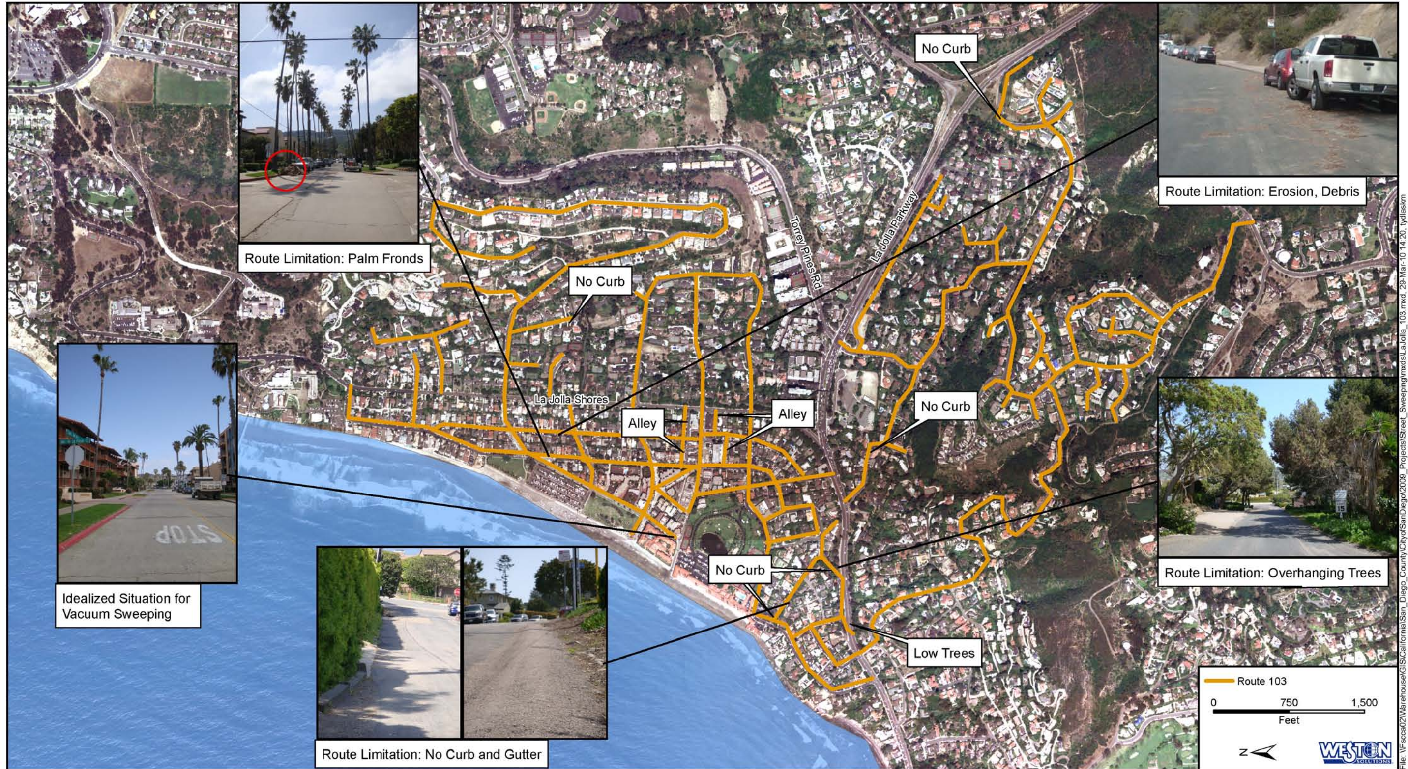
Figure 2-4. Close Up of Route 103 in the Commercial and Residential Areas of La Jolla Shores with Noted Route Limitations for the Vacuum and Regenerative-Air Sweepers
