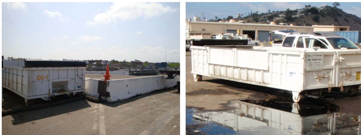
Figure 2-9. Concrete Ramps at Chollas Creek Service Yard (left) and Bin Structurally Modified to Include a Side Gate at Rose Canyon Operations Service Yard (right)
