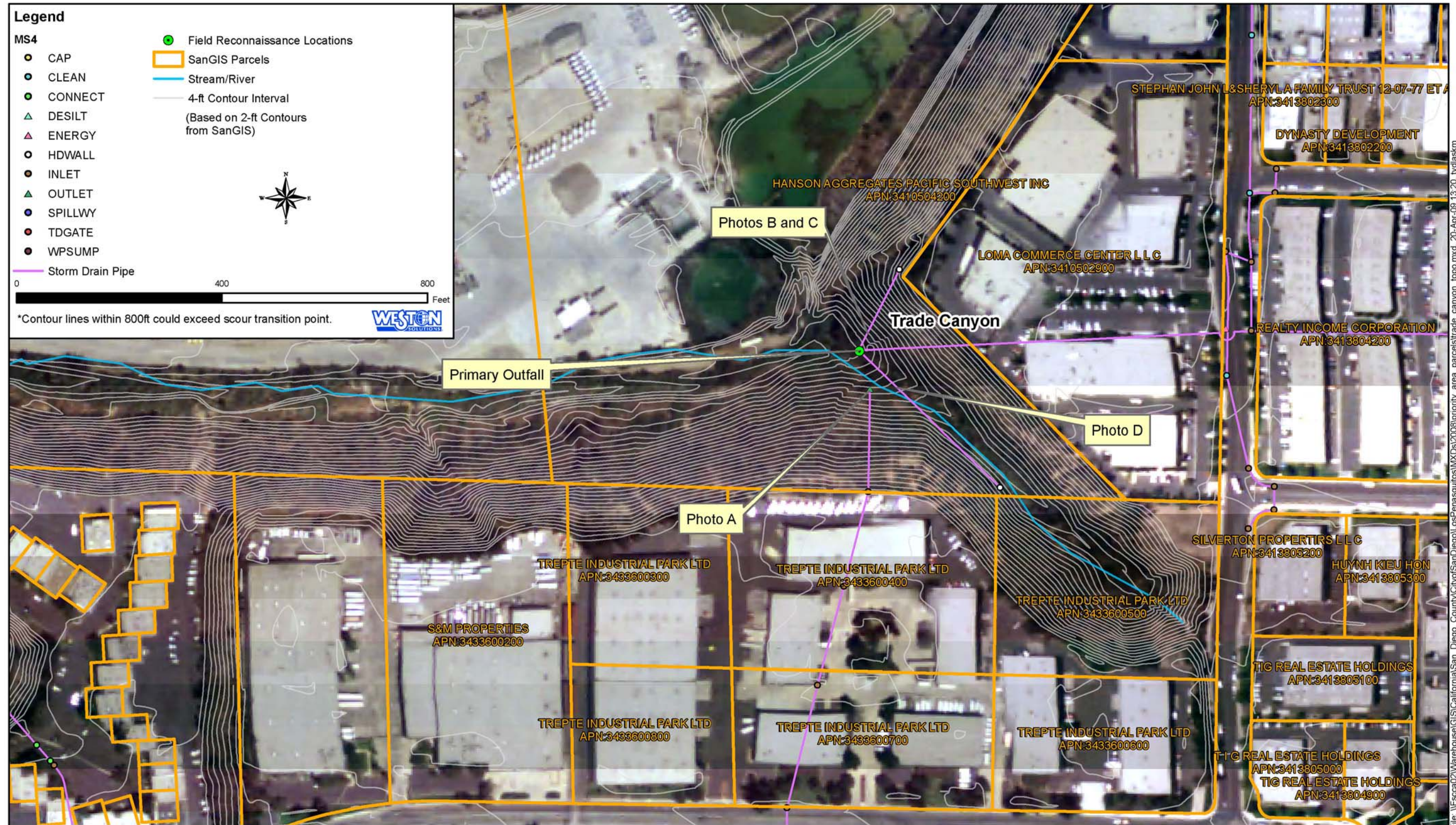
Figure 4-28. Topography and Photo Locations for Trade Canyon Outfall
