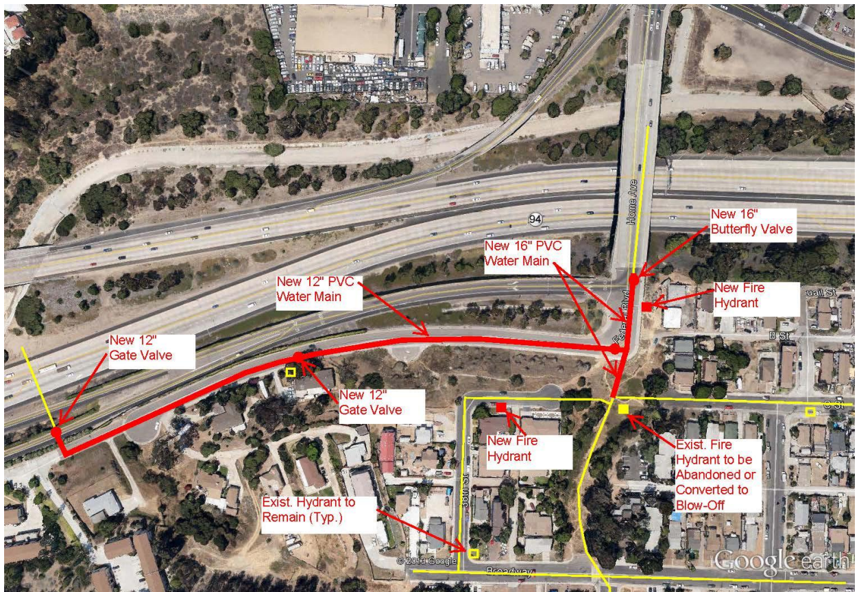
Exhibit 1 – Proposed Water System Improvements along Federal Blvd. (South)
