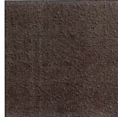
S-4 EXTERIOR CEMENT PLASTER SMOOTH FINISH INTEGRAL COLOR: MOON SHADOW
