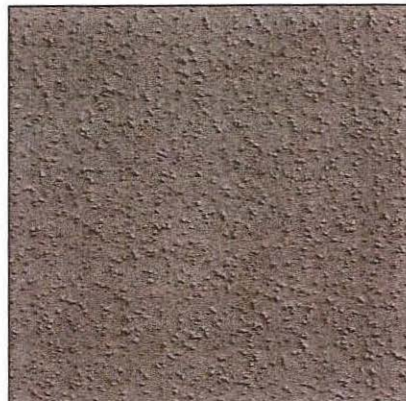
S-2 EXTERIOR CEMENT PLASTER SMOOTH FINISH INTEGRAL COLOR: MORROCAN SAND
