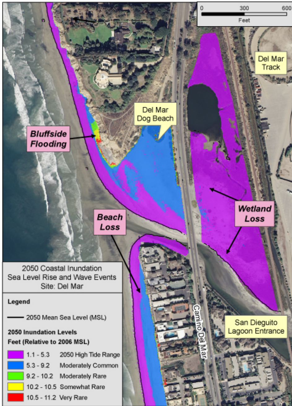
Figure 3-10. 2050 Coastal Inundation: Del Mar Beach. Tidal fluctuations alone (purple) appear to inundate much of sandy beach and entrance to San Dieguito Lagoon. Adding run-up from moderately common wave events (blue) floods majority of sandy beach (Dog Beach) and causes bluff-side flooding. Very rare wave events (red) flood sandy beach, cause bluff-side flooding and may impact coastal homes. The more frequent exposure of the base of the bluffs to waves on high tides increases the likelihood of bluff failures.
