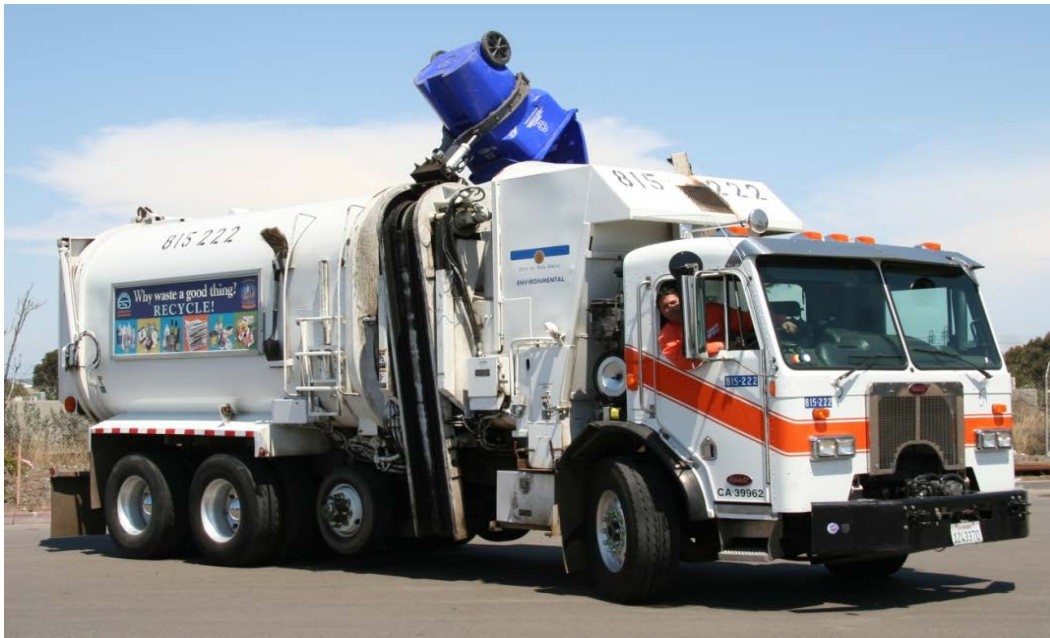
An automated refuse packer used by the Environmental Services Department. Photograph from City of San Diego archives.
