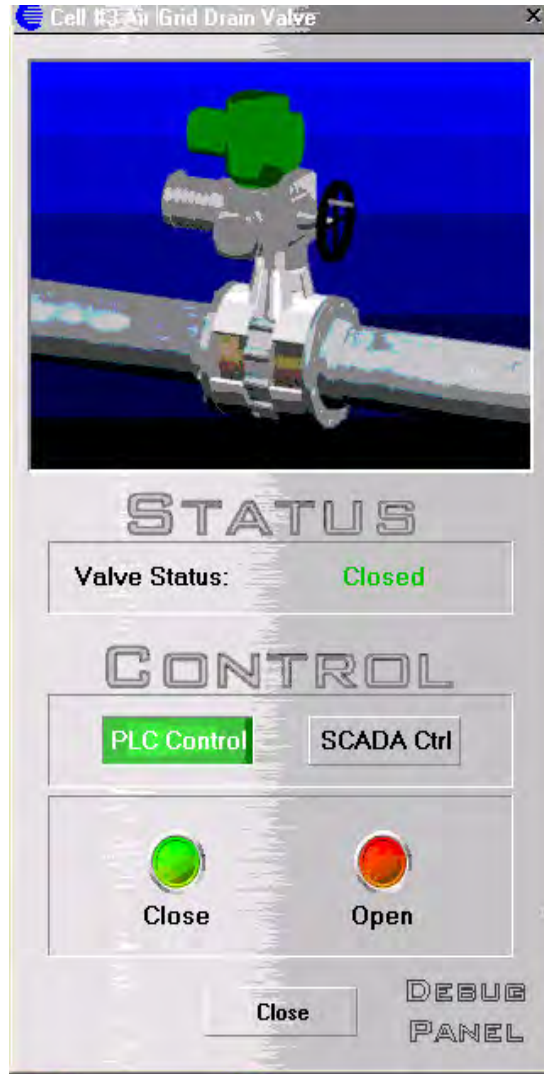
Figure 1. SCADA Inset Showing Control Switches For Individual Equipment.
