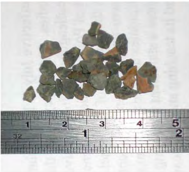
Picture 4. Top. Upper sight glass on the Biostyr, showing media. Picture taken during media loading. Bottom: details of media- reddish brown – Biofor, white Biostyr.
