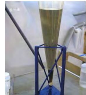
Figure 3.6. Photo of Backwash Sample Settling in Imhoff Cone
