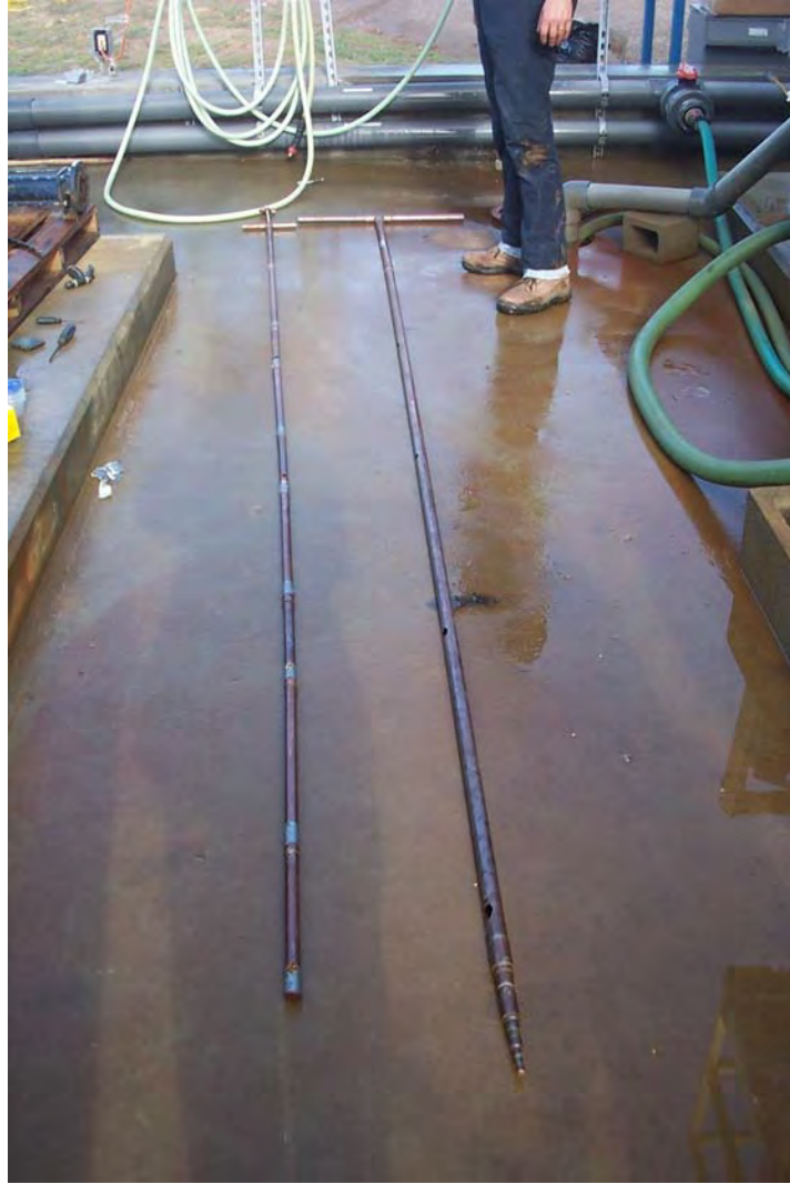
Figure 4.40. Photo of Media Sampler Used to Collect Biostyr Media at Discrete Depths
