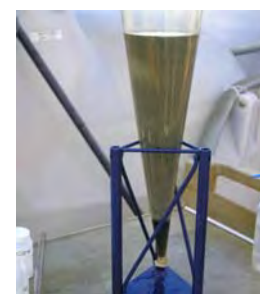
Figure 4.23. Photo of Sample Settling in Imhoff Cone
