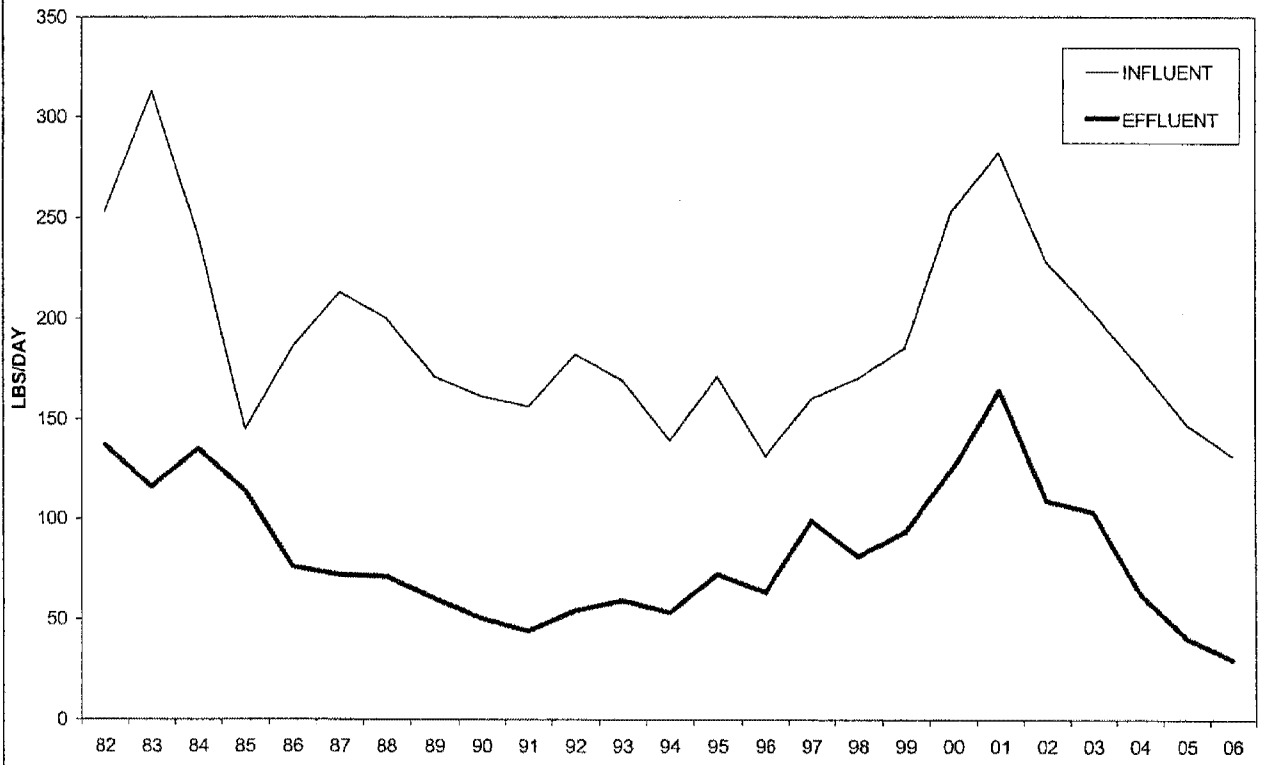
FIGURE 5.2-4 PT LOMA WASTEWATER TREATMENT PLANT - COPPER
