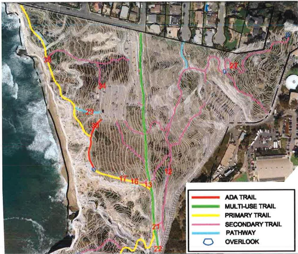
Figure 39. Shows preliminary Park Trails and the locations of erosion that will affect the Park Trails. The red numbers refer to Figures that discuss and show the erosion problems. The effects of erosion need to be considered in trail design and engineering.
