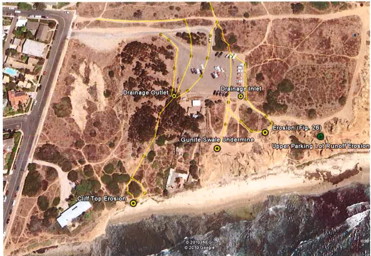
Figure 26. Pathways runoff follows (shown in yellow) before runoff enters and after it leaves the Lower Parking Lot. Very little parking lot runoff passes through the existing Lower Parking Lot drainage system (in the southwest corner). This drain should carry the runoff to the discharge and the Gunite swale, seen as a light colored feature running across the bowl shaped area in the center of the picture.
