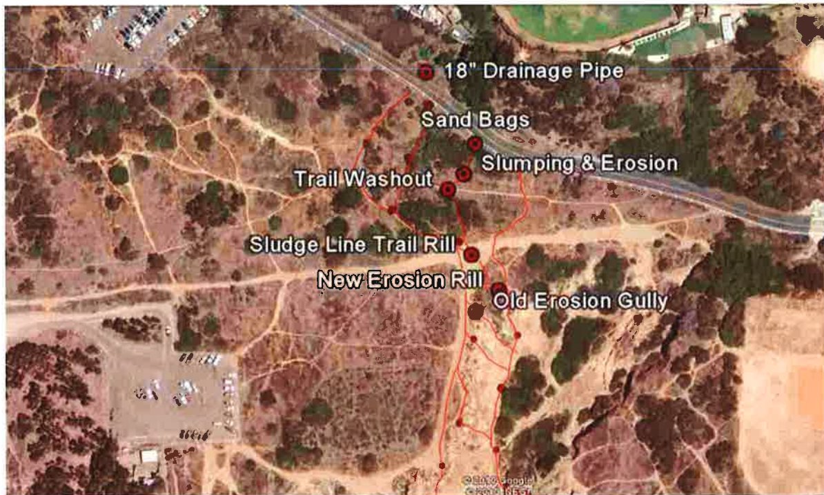
Figure 6. Runoff and erosion features associated with the 18" PLNU drainage pipe that discharges onto the Loop Road at the marked location. The large red dots show the location of features, and the small dots and streamlines show where evidence of watercourses transporting runoff that ponds on the Loop Road due to discharges from the 18" pipe can be seen after major rainfall events.
