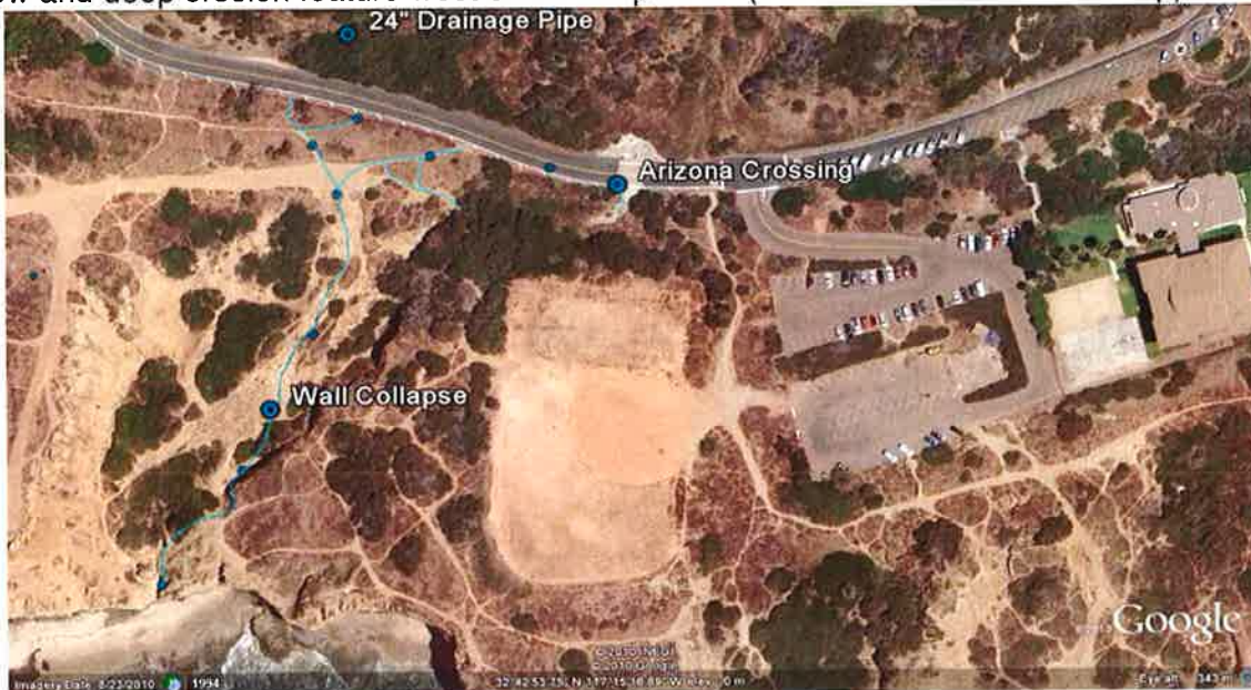
Figure 20. Erosion Caused by Discharges from the 24" Pipe to the Western Loop Road. For reference, the Badlands are on the left, Culvert Canyon is the deep feature to the left of center, and the old ball field is to the right. Runoff from the 24" pipe flows over the Loop Road curb and into the southeast corner of the Badlands and Culvert Canyon at locations indicated by blue dots. Runoff across the Park roughly follows the blue streamlines showing the linkage between erosion on the sludge line trail and the wall collapse area in Culvert Canyon. During periods of high flow the runoff also flows over vegetated areas.
