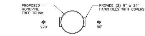
A POLE PLAN AT LOWER HANDHOLES @ 3'-0"
