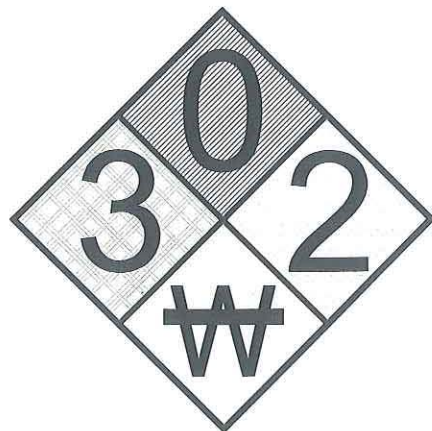
REQUIRED NFPA SIGNAGE
