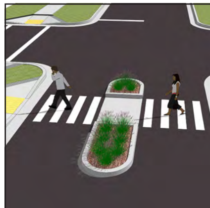
Median Refuge (Use with SC.3 Pedestrian Crosswalk)
