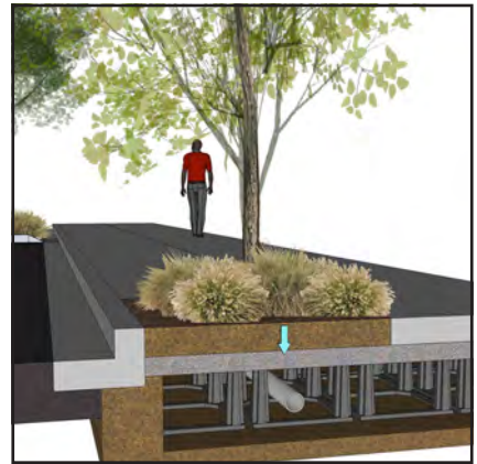
Subsurface Silva Cells & Drain (Use w/ Permeable Surface)
