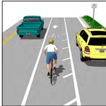
Class 2 Bike Lane with Inside Buffer
