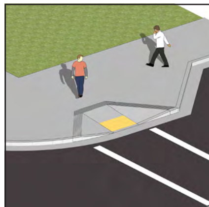
Pedestrian Ramp & Bulbout (Midblock or Intersection)
