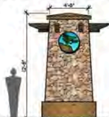
OPTION 'C' LARGE MONUMENT PILASTER (SECTION) (FIELDSTONE)
