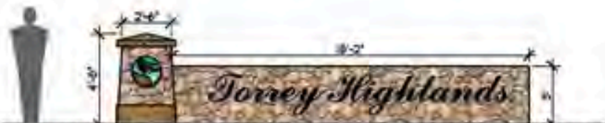
OPTION 'C' SMALL MONUMENT PILASTER & SIGNAGE WALL (SECTION) (FIELDSTONE)
