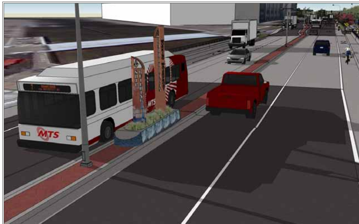
A support base would be designed to divert vehicles from collision impacts to the structure and for driver safety
