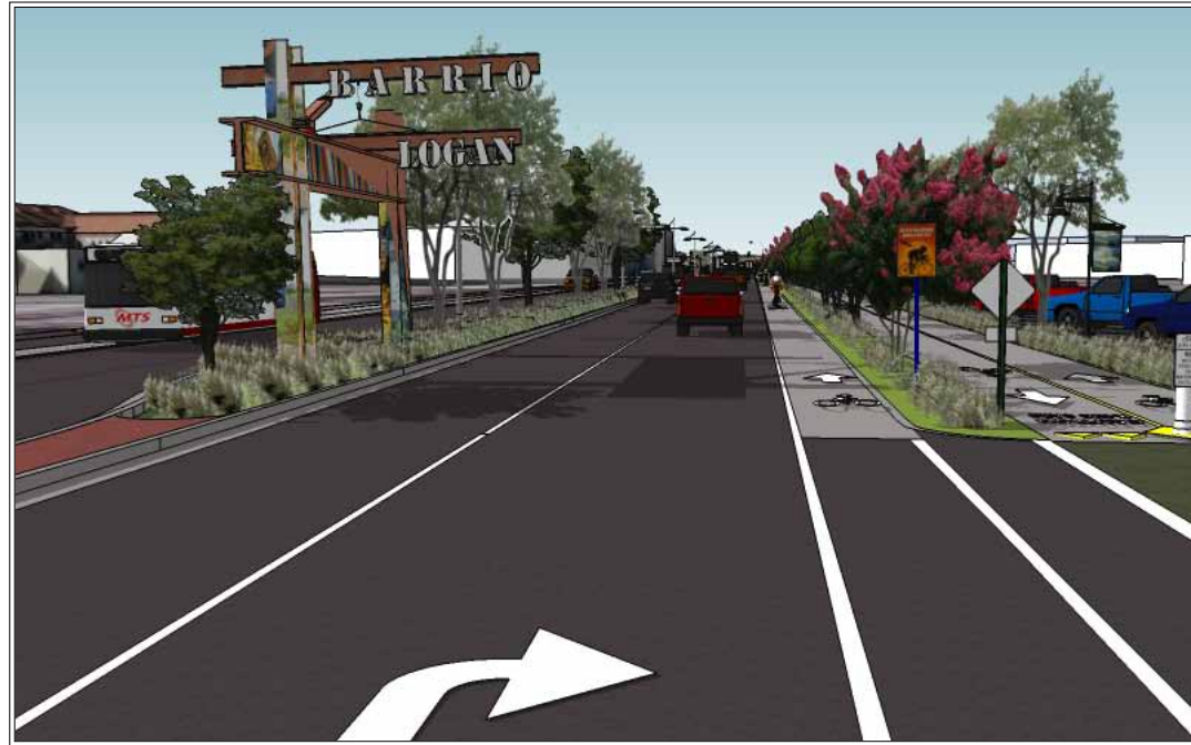
Barrio Logan cut-out letters that overhang Harbor Drive with a minimum of 15' clearance
