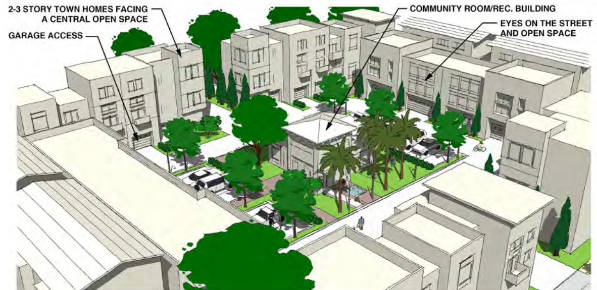
FIGURE 4-9: Building Orientation to Open Space
