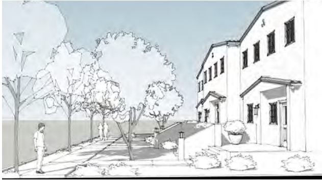
Figure 4-4: Building Frontage Type - Stoops are appropriate in El Pueblito Viejo Village, Sunset Neighborhood, Beyer Hills Neighborhood, and San Ysidro North Neighborhood
