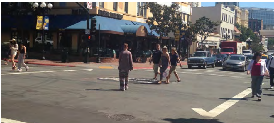
Example of scramble pedestrian crossing intersection
