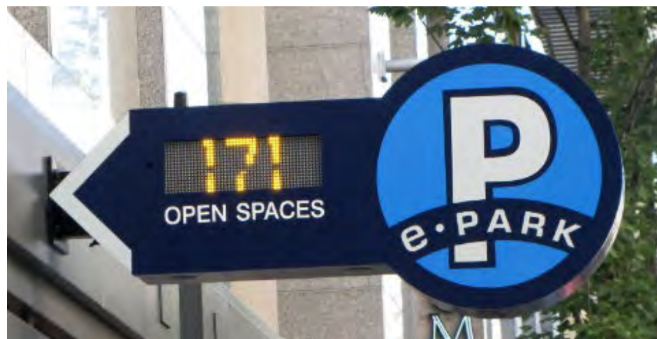
Real time parking information at this parking garage provides the number of spaces available and can be linked to a smart phone for efficient access to parking.
