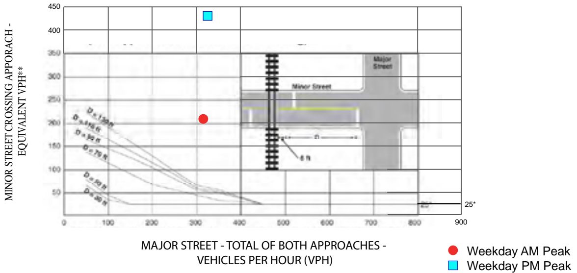
Figure 4C-10. Warrant 9, Intersection Near a Grade Crossing (One Approach Lane at the Track Crossing)
