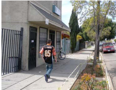
Narrow sidewalk conditions that do not meet Americans with Disabilities Act (ADA) requirements correspond to worse LOS values, such as on Commercial Street (top). Where sidewalks are present and the separation of pedestrians and traffic is adequate, as shown on National Avenue (bottom), pedestrian LOS values are more acceptable.
