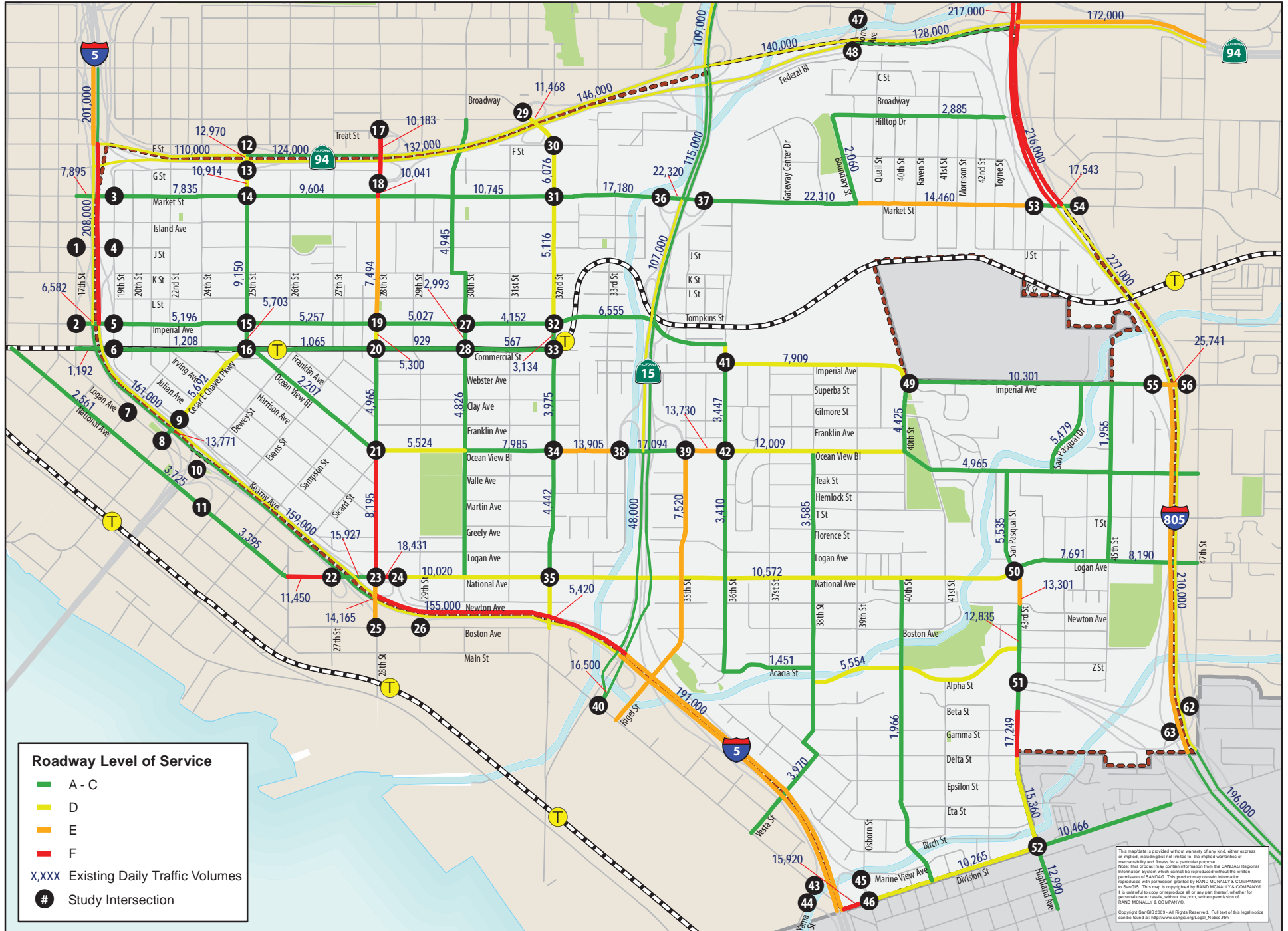
Figure 3-14: Existing Roadway Traffic Volumes and Level of Service
