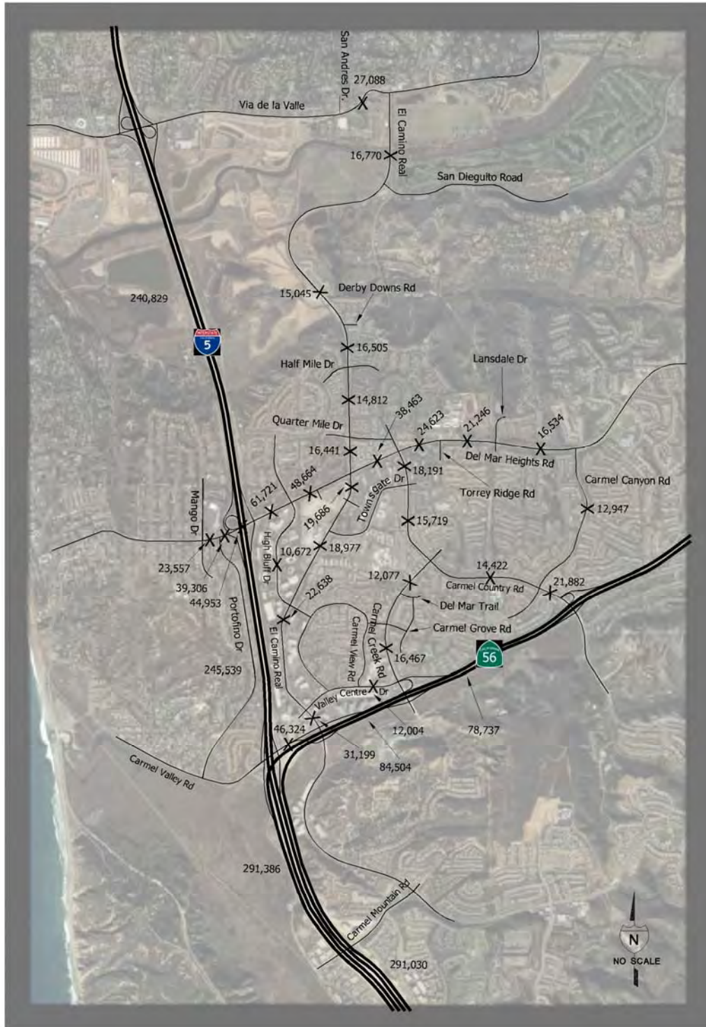
FIGURE 10-1 Near Term With Project Average Daily Traffic (Phase 1 & 2)
