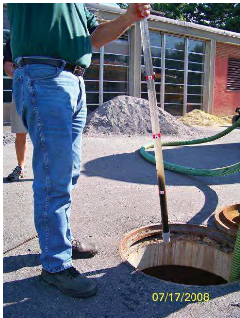
The depth of sediment and oil can be measured from the surface by using a sediment probe or dipstick tube equipped with a ball check valve and inserted through the 30-inch maintenance access pipe. This large port provides convenient access for inspection and vacuum removal of water and pollutants.
