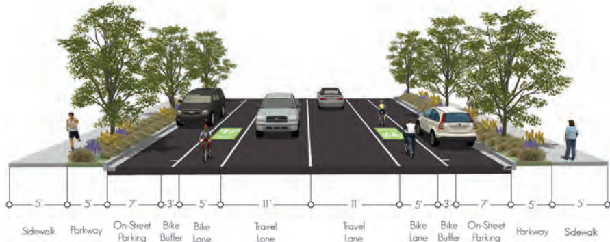
Figure 3-13: Example of Bicycle Focus Green Street Design applied to a 72 ft. ROW
