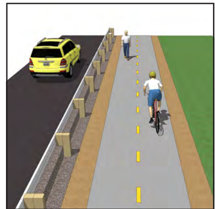
Two-Way Cycle Track with Barrier
