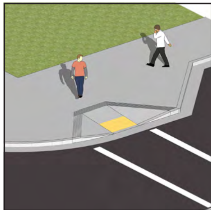
Pedestrian Ramp & Bulbout (Midblock or Intersection)
