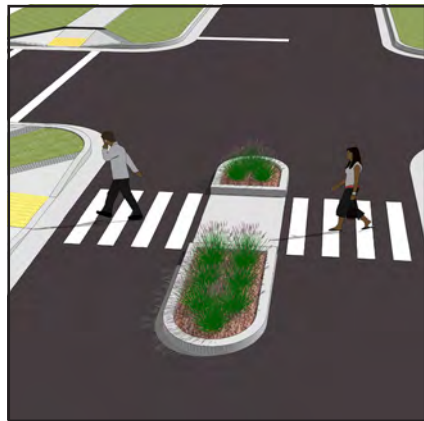
Median Refuge (Use with SC.3 Pedestrian Crosswalk)
