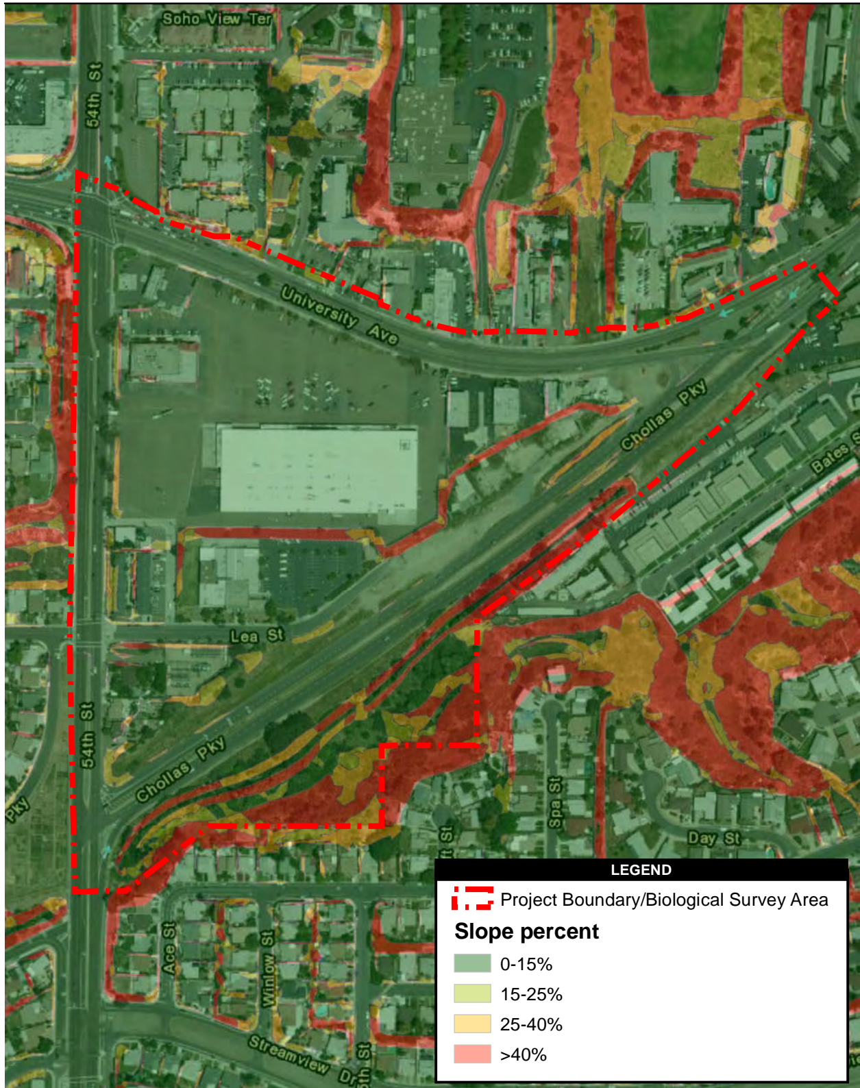
Figure 7 Step Slope Analysis
