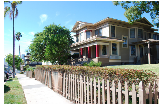
A generous front porch and canopy tree effectively manage solar heat gain on this residence.
