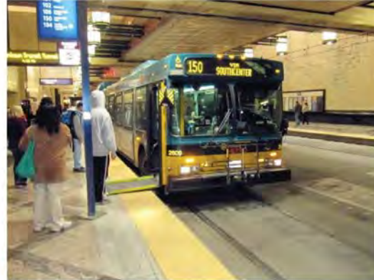
Buses and light rail sharing a 14 in. platform in Seattle, where special mitigations have been applied (pavement ramp adjacent to platform edge and larger tires on bus).
