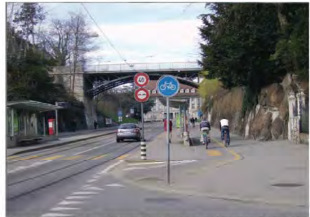
Bern, Switzerland: Bicycles are routinely routed onto the sidewalk to bypass tram stops, but policy states that this is only appropriate on uphill grades.
