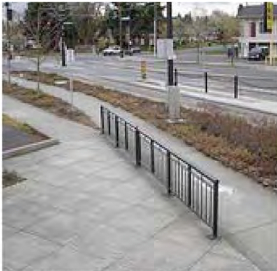
Bicyclists are directed off the street and onto a separated bike path in order to cross the tracks at a right angle at this Portland MAX stop.
