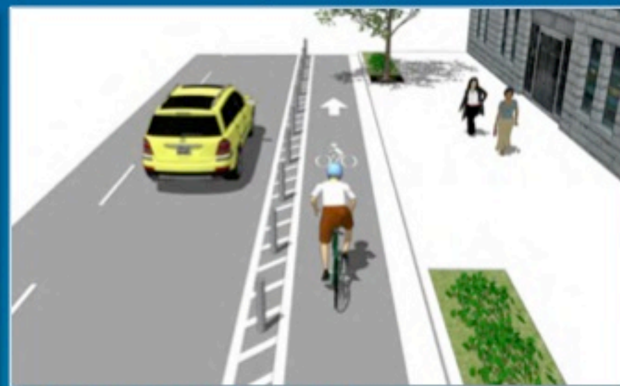
Cycle Track (one-way with bollards)
