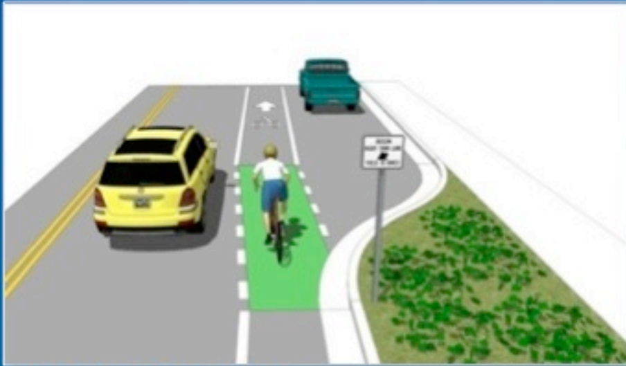
Class 2 Painted Crossover Lanes
