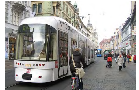
This example of a shared road allows equal access and priority to trains, cars, and pedestrians without the use of curbs. Subtle design features such as material change or color visually indicate pedestrian areas.
