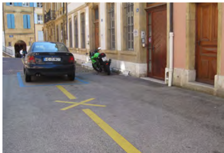
Using paint striping or alternate materials to designate parking and pedestrian areas could help to improve pedestrian safety and preserve parking and rail access without constructing sidewalks and curbs.
