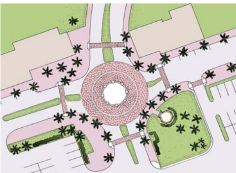
Above photo: Fort Pierce, Florida. This roundabout eliminated a four lane roadway, tamed traffic entering downtown Ft Pierce, and created an attractive gateway to the shopping district.
