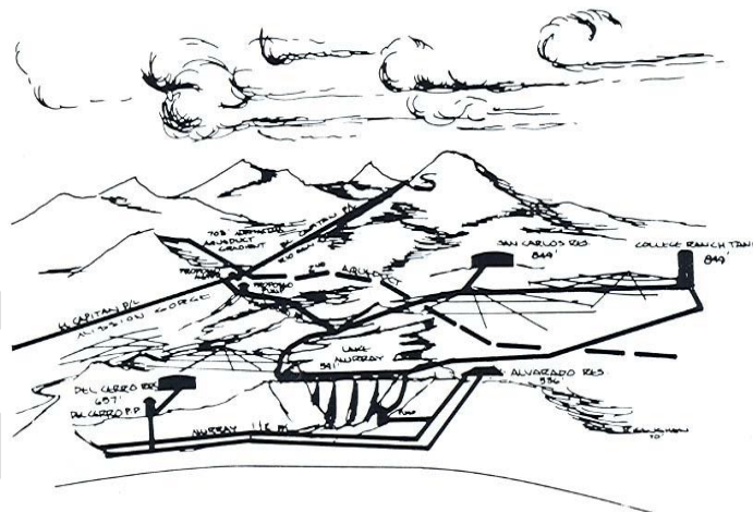
SCHEMATIC VIEW OF SAN CARLOS WATER SYSTEM
